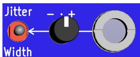
Just on top of the **Width knob** there is a control voltage CV input directed to an **attenuverter** and going into
