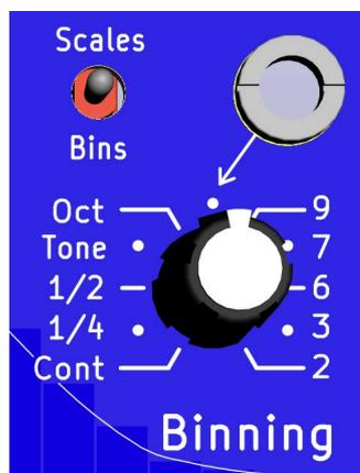
There is a **switch** with two states **Bins** and **Scales**, it allow to adress the type of quantisation of the **CV outputs**, it works together with **Binning knob**.
