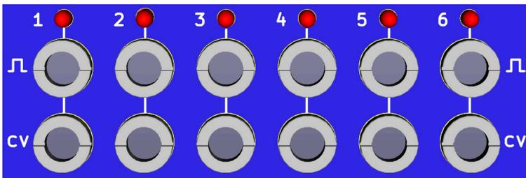
For each of the six **GATES Outputs**, there is a corresponding control voltage **CV Output**. The CV levels are changing synchronously to the corresponding gates rising edges. The algorithm used to generate these control voltages is using a gaussian distribution controlled by the knobs sitting on the top of the module panel. The gate LEDs let you monitor the pulses width and/or when the CV value is being updated.
