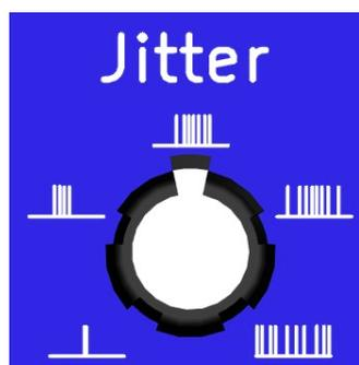
The **Jitter knob** adds a time offset (time delay) to each of the six **Gate output** with respect to the main clock (external or internal). This jitter could be generated both before/after relative to the main clock tick. At each input clk edge the algorithm compute the next coming clock jitter combinaison to be applied. So always expect 1 clock cycle delay to get the result of the variation of a module parameter.
