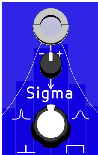
The **Sigma knob** adjusts the width parameter of the Gaussian distribution.
