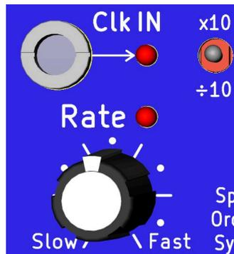
The **Rate** controls the period of the internal clock generator of the module. It works together with the multiplier switch [x10 x1 /10] to reach a wide range of periods from 10ms to 20s. The associated **Rate LED** helps to monitor the actual rate.
