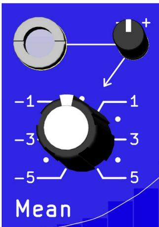
The **Mean knob** setting correspond to the mean value of the distribution of outgoing CV levels. It can be interpreted as a global offset of the six **CV outputs** level around which gaussian voltage variations will be added.
