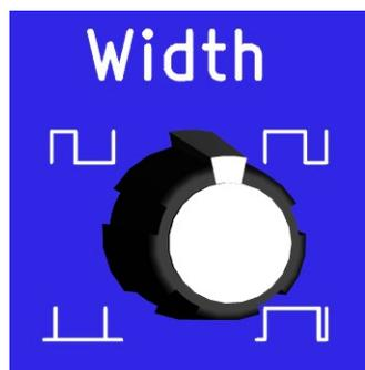
The **Width knob** controls the duration (duty-cycle) of the generated Gate Pulses. It is set in percentage of the main clock cycle. So when the clock rate changes the pulse width will follow accordingly. The smallest Gate width is 1% of the duty cycle, the maximum width is 99%.
